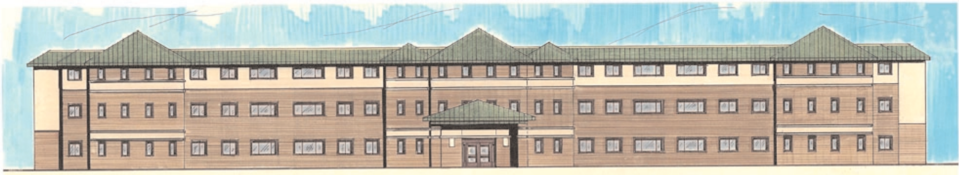
Scheme B: 1. Green metal roof to add color and interest to building. 2. Hipped metal roof added to existing canopy for prairie school look. 3. Front doors replaced with glass double doors with sidelights. 4. Hipped roof eaved on building roof over center and bumped out end sections. 5. Horizontal stone banding added to break up vertical spans. Cost estimate: $300,000
