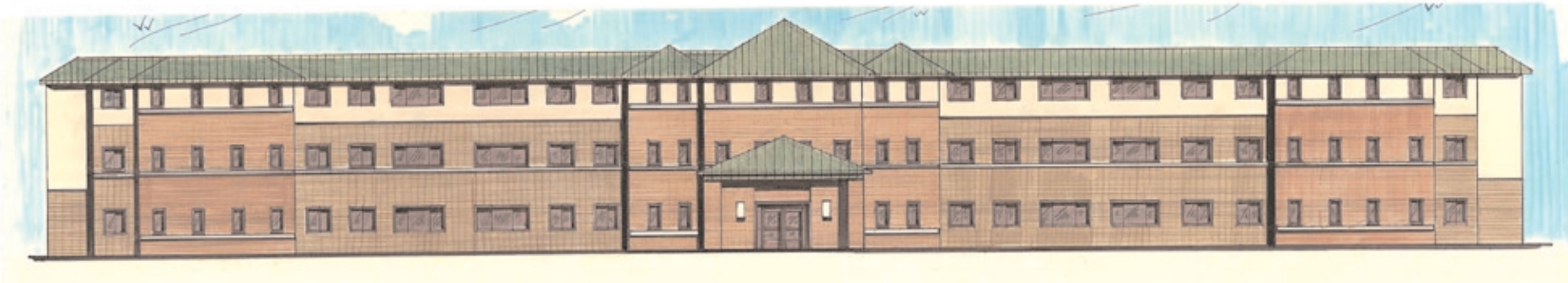
Scheme A: 1. Green metal roof to add color and interest to building. 2. Hipped metal roof added to existing canopy for prairie school look. 3. Front doors replaced with glass double doors with sidelights. 4. Hipped roof eaved on building roof. 5. Horizontal stone sills added to break up vertical spans. Create more horizontality. Cost estimate: $275,000
