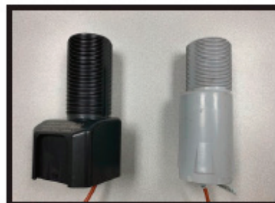
New Orion (left) v Old Orion (right) weather shields removed
